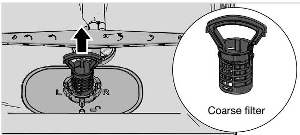
1. Lift the coarse filter by the handle.
