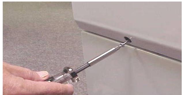
9. Reinstall the hole plugs removed in step 2.
