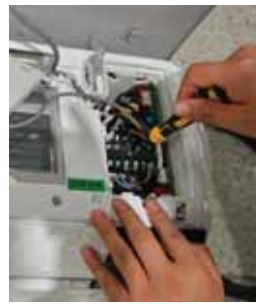
4. Remove 1 screw to remove the terminal block (GS06WP2BE* models only).
