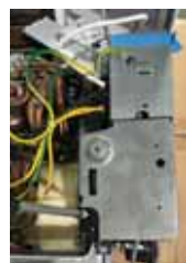
4. Remove the electrical box cover.
