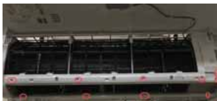
2. Remove the screws.
