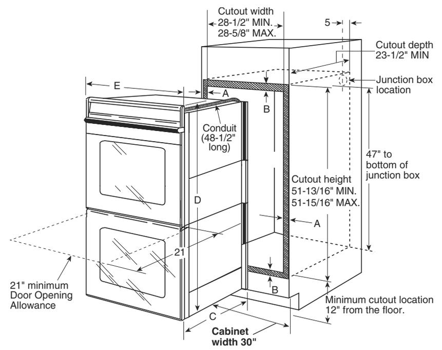
MOST 30" WALL CABINETS CAN BE USED WITH THIS UNIT. THE OPENING BETWEEN THE INSIDE WALLS MUST BE AT LEAST 28-1/2" WIDE.
