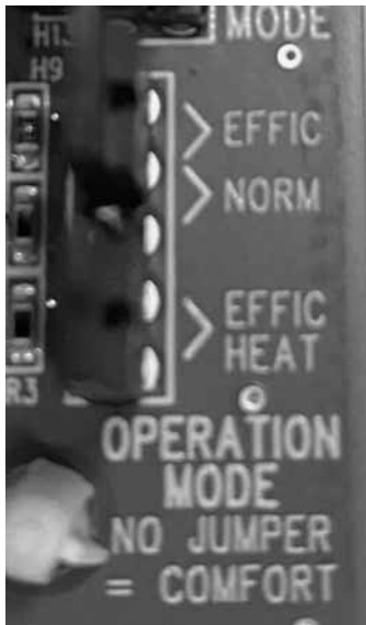
Figure 45. Operation Mode Jumper
