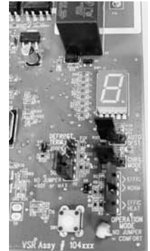
Charge Mode and Operation Mode Jumper Detail
