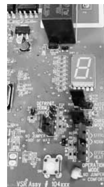
Charge Mode and Operation Mode Jumper Detail
