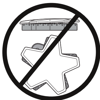
Incorrect burner cap
