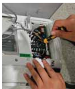
4. Remove 1 screw to remove the terminal block (QS06WP2BE* models only).
