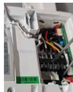
4. Remove 1 screw to remove the terminal block (QS06WP2BE* models only).
