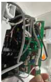
5. Pull out the PCB and unplug the refrigerant leak sensor from CN3.
