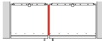
EN: When the appliances are installed less than  $6\frac{1}{4}''$  (160 mm) apart from one another, but not connected side-by-side, purchase the heater kit **HEATRKIT20** (Freedom Heater Kit). This kit is also recommended for use with any installation in areas that are subject to extreme humidity.
