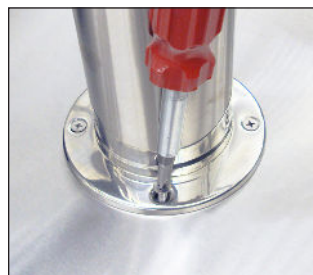
FIG. 3. Secure the draft standard to the countertop.
