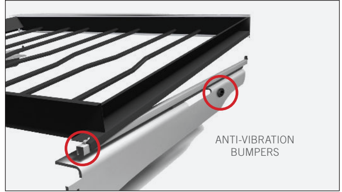
FIG. 2. Be sure the anti-vibration bumpers are on the hinged side.
