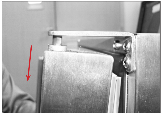
FIG. 3. Lower the door off the top hinge.
