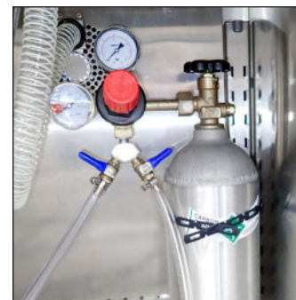
FIG. 9. Always strap the CO 2 cylinder into the appliance.
