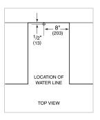
ICE MAKER DRAIN lce maker models can be ordered with or without a drain pump. Models without a pump will drain water by gravity. A drain must be provided for all models.
