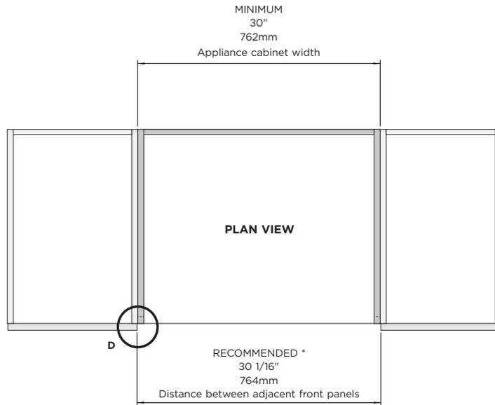
\*NOTE: Dimensions based on 1/16" (1.5mm) clearance between Drawer and adjacent panels. Product widths vary, consult detail views D1 and D2 for Oven and Coffee Maker or Cook Product clearances.
